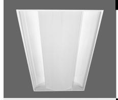
Provides indirect, soft, uniform illumination. Curved perforated details combine recessed fixture advantages with efficient indirect shielding. Perforated center basket, backed with reflective white acrylic, controls glare and veiling reflections. Shielding is easily removed for relamping. Optional Side Lenses improve visual comfort and prevent dust from entering the lamp chamber. Flanged fixture available for plaster ceilings.
