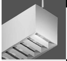
Available in nominal lengths up to 8'-0" sections, 1 lamp T5 or T8 operation, custom lengths available upon request. For continuous runs please consult factory with specific wiring instructions. Simple clean linear lines allow for this fixture to blend aesthetically into almost any space. Mounting can be accomplished using adjustable aircraft cables or rigid stems. Wall mount is also available.
