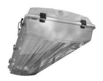
Standard with stainless steel latches. For pendant mounting. Stainless steel mounting brackets reduce installation time and eliminate the need for mounting holes in fixture body. Stainless steel V hooks simplify pendant mounting with chain or cable. For individual or continuous row with flexible conduit.
